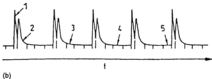
FIG. 13b Elution diagram showing the automatic separation of fullerene raw material obtained by Soxhlet extraction of carbon soots with hexane. Injection frequency, 8 \text{ min} ; detection, UV at 350 \text{ nm} . Conditions: two columns ( 600 \times 20 mm i.d.) in series + 60 \times 20 i.d. guard column; stationary phase, PSS-Gel ( 10 \mu\text{m} , 500 \text{ \AA} ); mobile phase, toluene at 15 \text{ mL/min} ; injection, 7.5 \text{ mL} of a saturated solution of fullerene raw material in toluene. Reprinted from Gügel et al. (52), copyright 1993, with kind permission from Elsevier Science Ltd.
